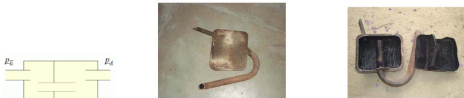
Fig.1.1 Reflective Muffler. Reflective muffler in closed condition Reflective muffler in cut condition
