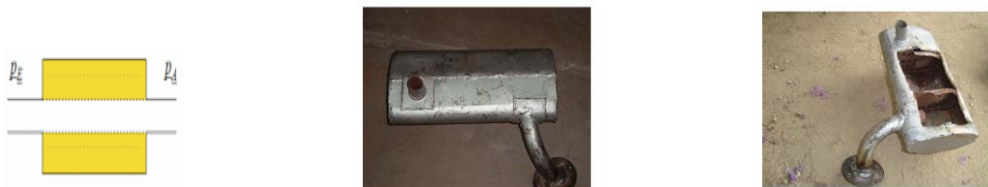
Fig.1.2 Absorptive Muffler Absorptive muffler in cut condition Absorptive muffler in cut condition
